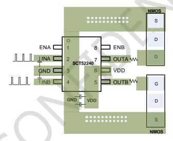
Figure 13. SCT52240 PCB Layout Example
