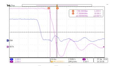
Figure 7. Driver Switching ON
