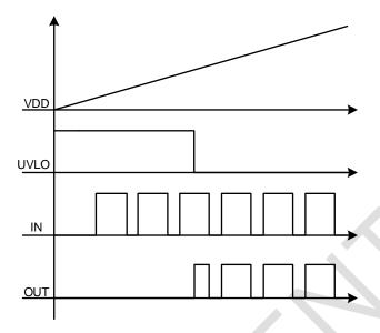
Figure 1 SCT52240 Output Vs VDD
