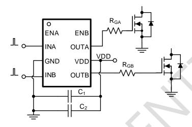
Figure 6. Dual Channel Driver Typical Application
