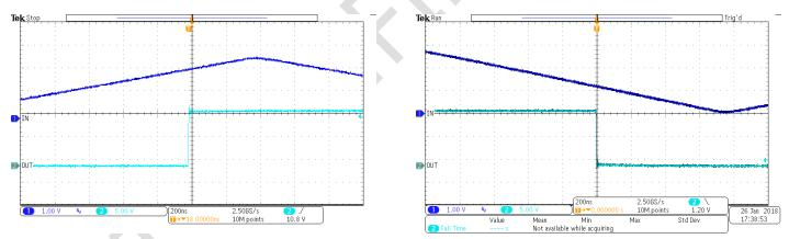
Figure 4. Driver Switching ON
