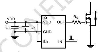
Figure 14. SCT51240 Inverting MOSFET Gate Drive Typical Application
